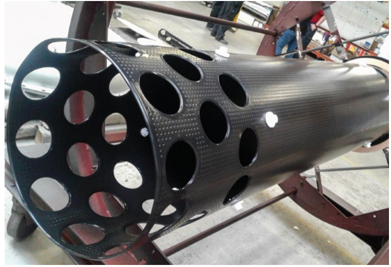
Process equipment with corrosion-protective Accoshield coating.
