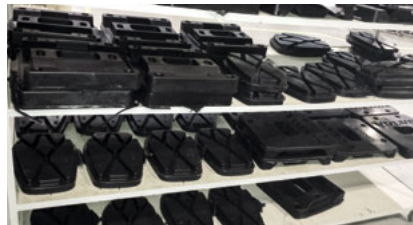
Volvo Pads for outriggers on excavators
