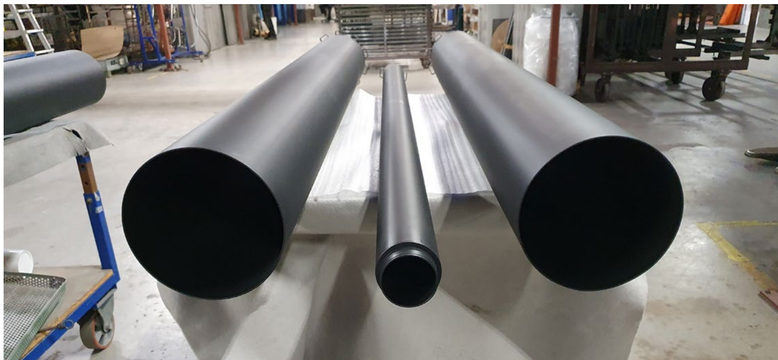
Pipes coated with P153 – a coating for non-stick and low-friction applications
