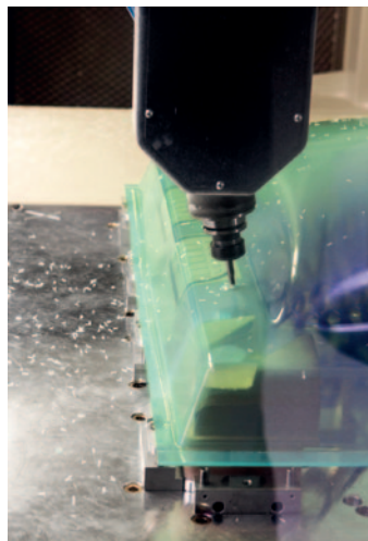
Trimming of a transparent part
