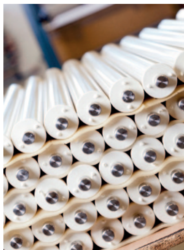
Rollers in hard PUR for developers (X-ray)
