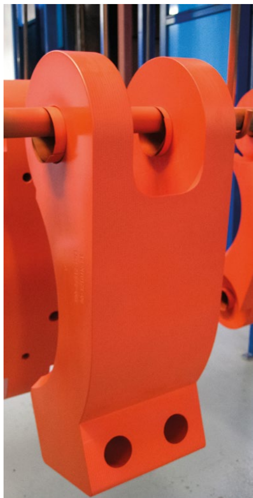
Clamps coated with Zylan
