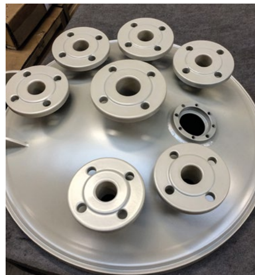
Tank top coated with Accotron BF
