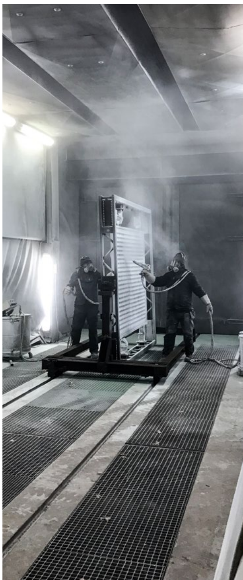
Accoat – coating with Accoshield powder
