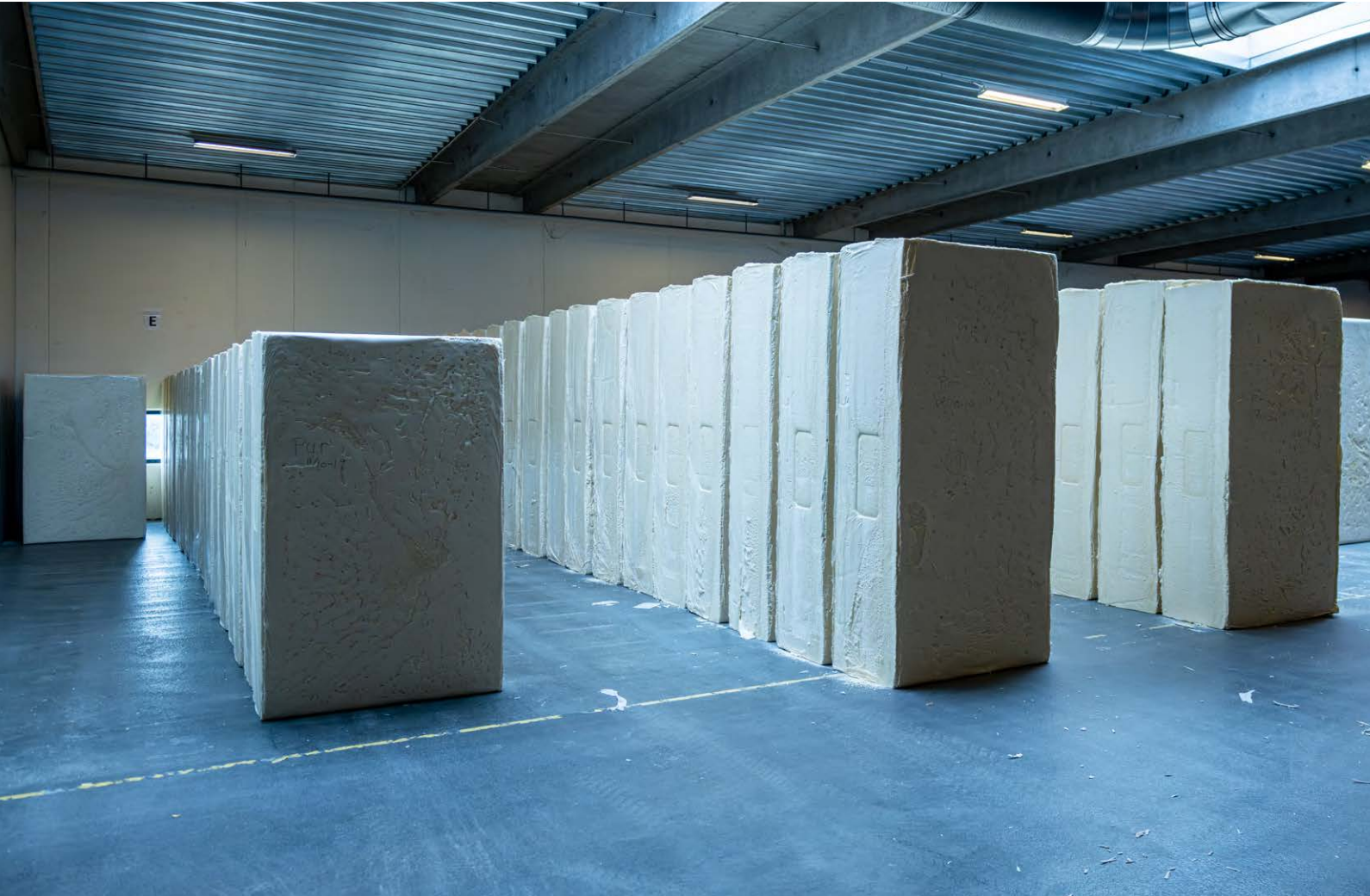
SP Tinby manufactures block foam made of PUR for insulation solutions for the construction and refrigeration industries.
