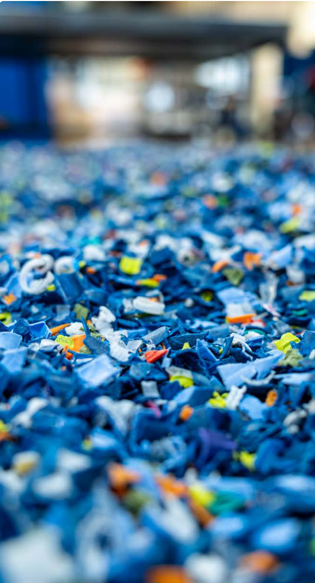
Collected consumer plastics are reprocessed into regrind material
