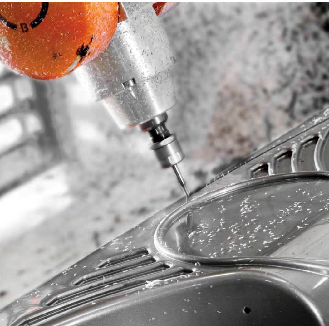
Plexx uses 5-axis simultaneous milling that facilitates machining of complex plastic components.
