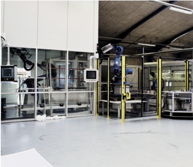
Automated production line for transparent vacuum formed plastic parts in dustfree environment
