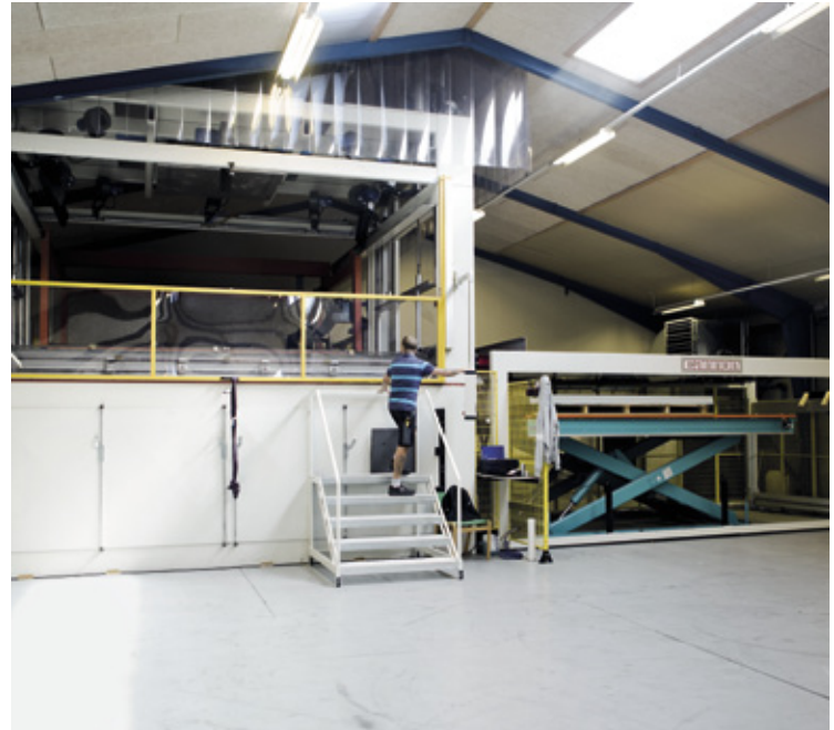
New large machinery – Vac421 that can produce components of up to 4.2 x 2.5 x 1.0 m
